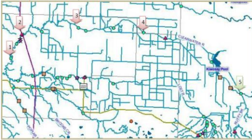
Figure 2. Clearwater River Nonpoint Study monitoring sites along the Clearwater River that led to the 303(d) listing of a dissolved oxygen impairment for this reach. Red arrows = partially or not supporting aquatic life. Green arrows = fully supporting aquatic life.
